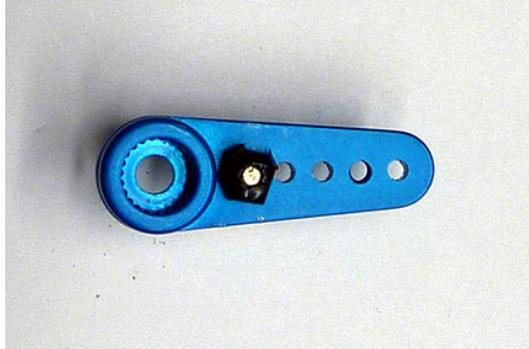
Trim plastic retainer of servo arm fitting to clear lip of splined shaft area and reinstall brass servo arm fitting. Make sure you remove enough material from plastic retainer to allow servo fitting to spin freely!
