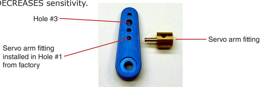
**Reference 2: Servo arm position when iTroll is at idle setting**
