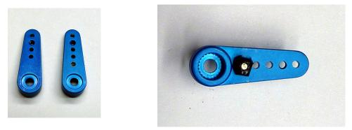
Trim plastic retainer of servo arm fitting to clear lip of splined shaft area and reinstall brass servo arm fitting. Make sure you remove enough material from plastic retainer to allow servo fitting to spin freely!
